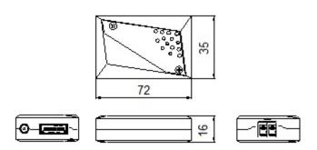
Note: The transmitter, DPFX-100-T and the receiver, DPFX-100-R have the same mechanical dimensions
