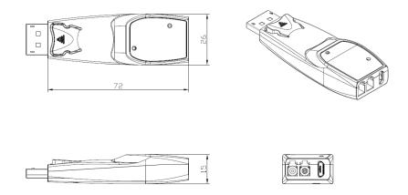
Note: The transmitter, DPFX-200-T and the receiver, DPFX-200-R have the same mechanical dimensions
