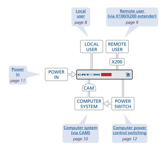
Connections do not need to be carried out in the order given within this guide, however, where possible connect the *power in* as a final step.
