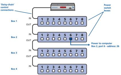
The power ports are connected to the power inputs of each computer system and the power switch box(es) are then connected to a mains power supply.
