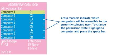
Here you can determine which of the connected computers can be accessed by the selected user account. Only computers that show the '+' marker to the right of the menu box will be accessible to the user account.
