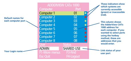
To view this menu at any time: Press and hold the hotkeys (usually  $\Box$  and A), then press M and finally release all three keys.
