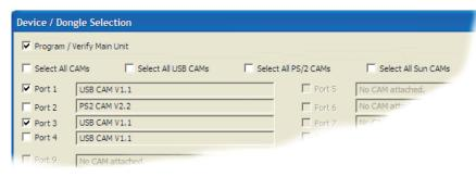
The type and firmware revision of each discovered CAM will be displayed alongside the port number to which it is connected.
