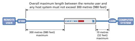
In situations where any computer system will be placed a significant distance from the AdderView CATx 1000 unit, ensure that the distance to any remote user is similarly less than 300 metres (980 feet).
