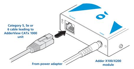
5 At the other end of the cable run, attach the cable connector to the socket on the front panel of the AdderView CATx 1000 unit.
