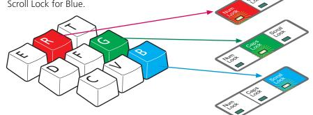
4 Press the ⊢ and ⊢ keys to retard or advance the timing of the selected colour channel respectively. On screen you will see a change in the position of the selected colour crosses (or colour bars) in relation to the other two.
