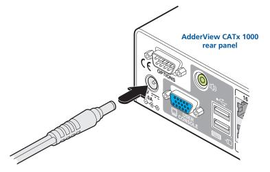
output lead from power adapter 2 Connect the IEC connector of the supplied country-specific power lead to the socket of the power adapter.
