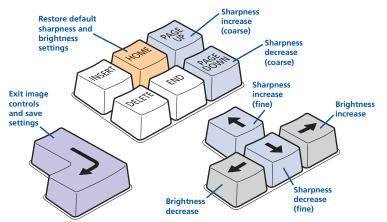
When no shadows are visible and the displayed images have crisp edges, press it o exit configuration mode and permanently save all settings.
