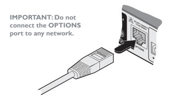
Note: If the optional CCS-XB module is used with the CCS-PRO, connect the computer instead to the **TO KEYPAD OR PC** port on the CCS-XB module.
