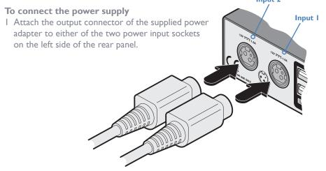
Note: The outer sleeve of each power connector will retract slightly as it locks into place.
