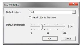
To impose a default colour on all connected indicators, choose the required **Default colour** and then tick the option **Set all LEDs to this colour**.
