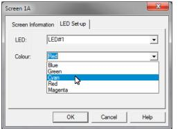
Note: Each LED indicator can only have one colour, so if you associate an indicator with more than one screen and then change the colour on a later screen assignment, it will be changed for all the screens in the list for that LED indicator.
