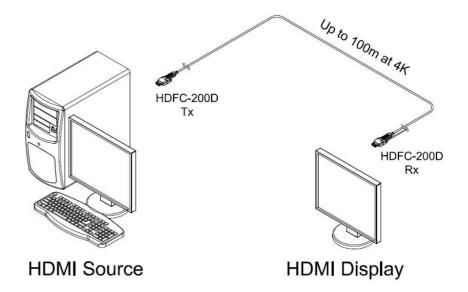
Figure 1 - General connection diagram of HDFC-200D
