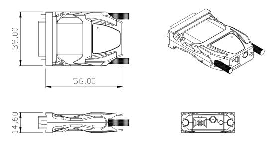
Note: The transmitter, DVFX-100-T and the receiver, DVFX-100-R have the same mechanical dimensions.
