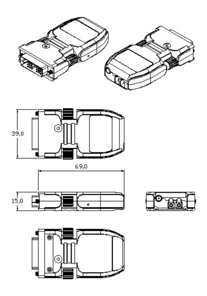
Note: The transmitter, M1-201DA-T and the receiver, M1-201DA-R have the same mechanical dimensions.
