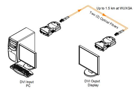
Warning; Dual LC patch cords made by some manufacturers could not fit in together since width of their plastic couplers are too wide to plug in M1-201DA-TR's LC receptacles. We recommend it to be 12.40 mm (not over 13.0mm).
