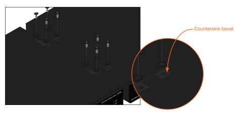
3 Turn the attached units over and install the included rack ears to one side of each enclosure using the included screws.
