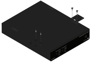
3 Mount the unit using the circular holes, on each mounting plate. If using a drywall surface, a #6 drywall screw is recommended. Mounting screws are not included.
