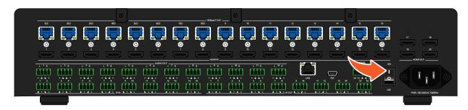
**NOTE:** If the matrix does not power, check to make sure that the power cable, on the rear of the unit, is connected to an active AC wall outlet. Also verify that the **ON/OFF** switch is in the **ON** position.
