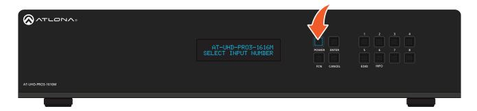
The matrix will power-down and be placed in a low-power state and the **POWER** button will be backlit by a solid red light.
