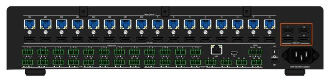
These four HDMI ports are used to mirror (copy) an HDBaseT output signal and duplicate it on any or all of these ports. By default, mirroring is enabled on these ports. However, mirroring can be disabled. When mirroring is disabled, any of the 16 HDMI inputs can be routed to these HDMI outputs, transforming this product into an 16 x 20 matrix switcher. The default mirror settings are listed below
