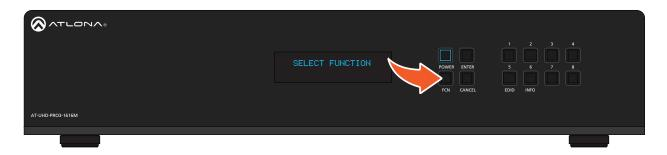
3. Press and release the **INFO** button to display the firmware version.
