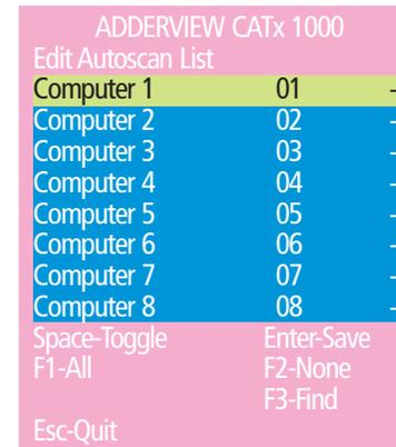
Cross markers indicate which computers will be accessible to the currently selected user. To change the permission state: Highlight a computer and press the space bar.
