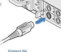
Connect the converter dongle locking 3-pin plug to one of the power outlets
