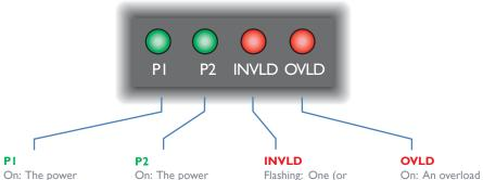
On: The power module in bay I has a mains input and is operating.
