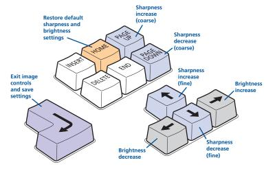
Sharpness: 1 U for fine adjustment, E for coarse adjustment.
