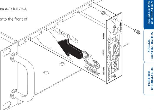
The naming of the LOCAL and REMOTE modules relate to their proximity to the computer system. Hence, the LOCAL module connects directly to the system, while the REMOTE is at the other end of the twisted pair cable and attaches to the keyboard, mouse, etc.
