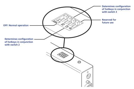
Note: When shipped, all switches are set in the OFF positions and this will produce normal operation.
