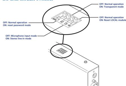
Note: When shipped, all switches are set in the OFF positions and this will produce normal operation with normal microphone input (at the REMOTE module).
