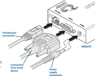
male connector on the REMOTE module labelled .....
