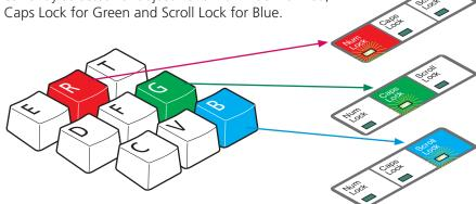
4 Press the 🗀 and 🔁 keys to retard or advance the timing of the selected colour channel respectively. On screen you will see a change in the position of the selected colour crosses in relation to the other two.
